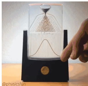
Figure: Galton Board (or quincunx, or bean machine): X = \sum_{i=1}^n X_i , where X_i \stackrel{iid}{\sim} \text{Bernoulli}(0.5) \in \{-1, 1\}
