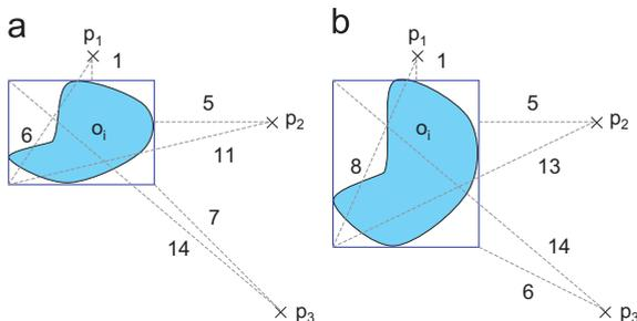
**Fig. 3.** Minimum and maximum distances for the min–max-dist pruning method. (a) An object with a relatively small uncertainty region. (b) An object with a relatively large uncertainty region.
