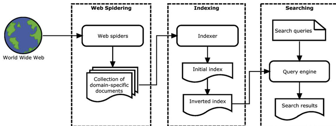
Fig. 1. Overall architecture of a common vertical search engine development tool.
